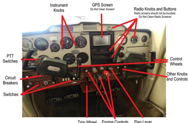
Trim Wheel **Engine Controls** Flap Lever **CESSNA 172S INSTRUMENT PANEL DISINFECTING DIAGRAM**
